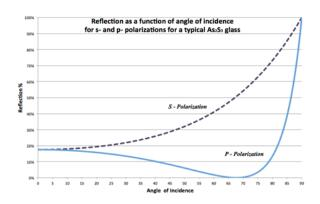
Figure 1: Reflection as a function of incident angle for S- and P-polarizations for an air-to-As<sub>2</sub>S<sub>3</sub> interface. It can be seen that for a certain angle the P-polarization experiences 0% reflection.
