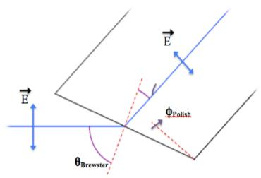
Figure 2: Diagram showing the input beam polarization for maximum transmission.
